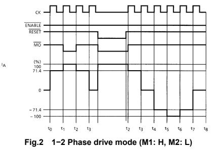
Low level active of  $\overline{\text{RESET}}$  Signal offs not only the Outputs but also stops internal CK functions and  $\overline{\text{MO}}$  to low. Outputs are initiated from the initial point after release of  $\overline{\text{RESET}}$  (High) as shown in Fig.2.  $\overline{\text{MO}}$  (Monitor Output) Signals can be used as rotation and initial signal for stable rotation checking.
