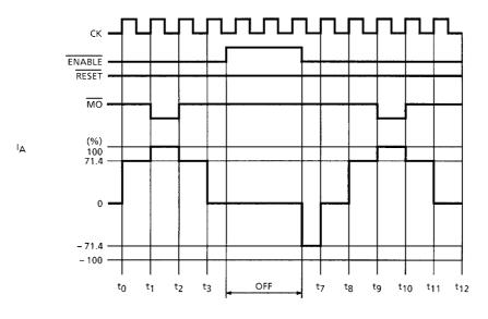
Fig.1 1-2 Phase drive mode (M1: H, M2: L)
